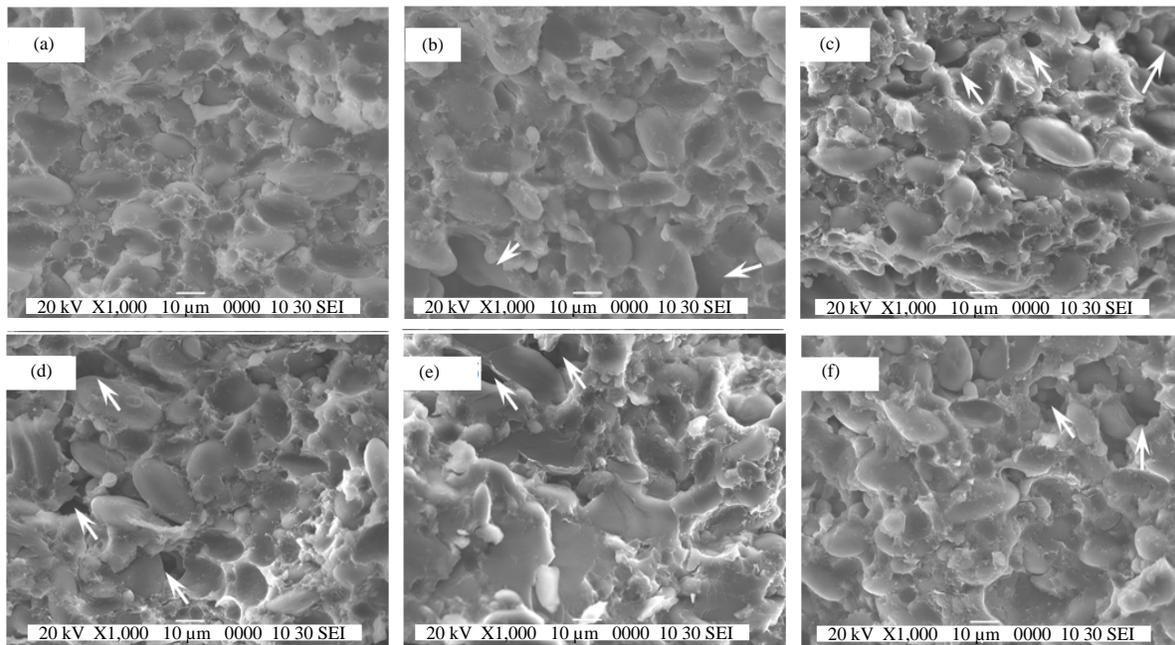
Fig. 3(a-f): SEM of dumpling wrappers with different PG contents after storage at  $-20^{\circ}\text{C}$  for 2 weeks (1000 $\times$ ), (a) Control, (b) PG5, (c) PG7.5, (d) PG10, (e) PG12.5 and (f) PG15
