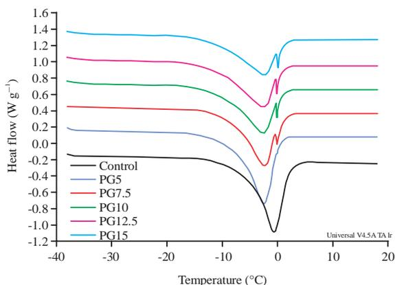
Fig. 2: DSC thermograms of dumpling wrappers with different levels of PG after storage at  $-20^{\circ}\text{C}$  for 2 weeks
