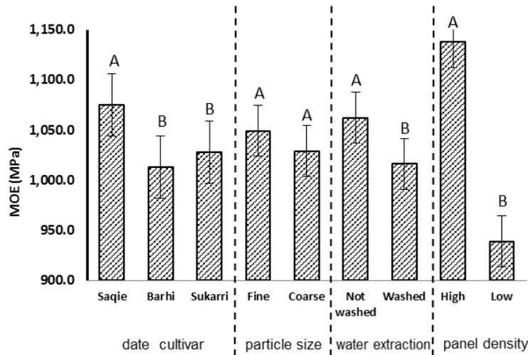
**Figure 6.** Effect of date palm cultivar, particle size, hot water extraction and panel density on Modulus of Elasticity (MOE) property. (Means with same letter do not significantly different at L.S.D.0.05).
