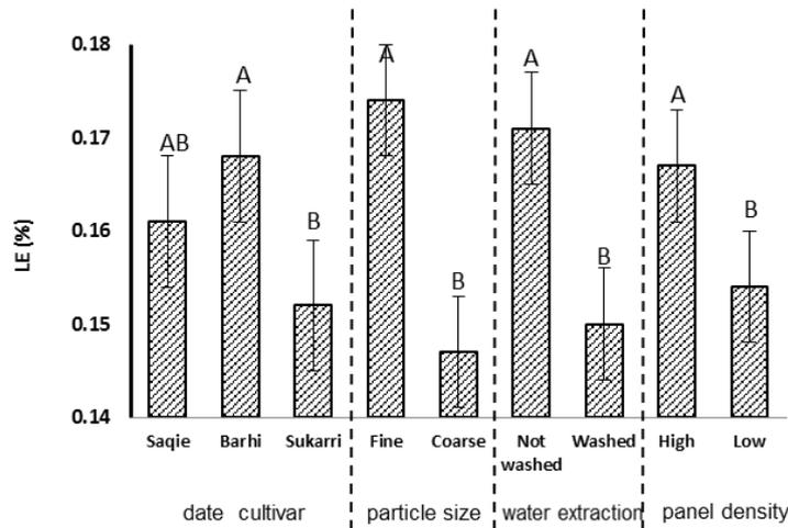
**Figure 8.** Effect of date palm cultivar, particle size, hot water extraction and panel density on linear expansion (LE) property. (Means with same letter do not significantly different at L.S.D.0.05).
