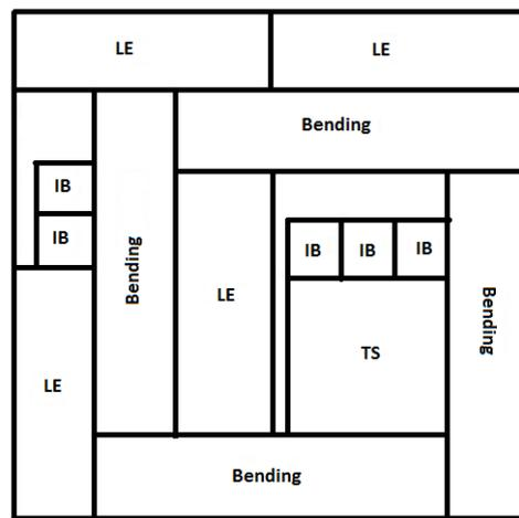
**Figure 2.** Cutting diagram for mechanical and physical samples taken from the manufactured panels (48 × 48 cm). Bending samples = 32 × 7.5 cm, internal bond (IB) = 5 × 5 cm, linear expansion (LE) = 24 × 7.5 cm, thickness swelling and water absorption (TS) = 15 × 15 cm.
