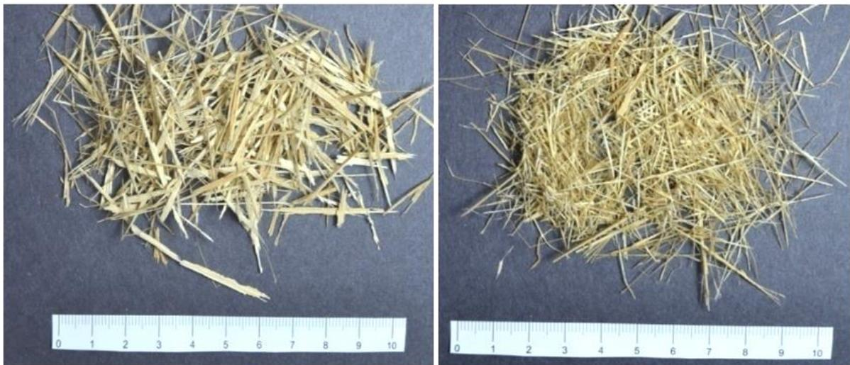
**Figure 3.** Coarse and fine date palm frond particles used in this study.
