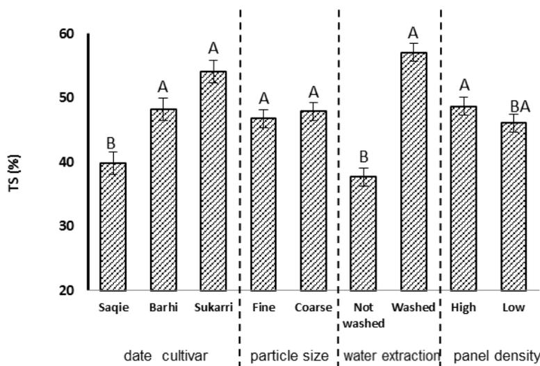
**Figure 9.** Effect of date palm cultivar, particle size, hot water extraction and panel density on thickness swelling (24-h TS) property. (Means followed by with same letter do not significantly different at L.S.D.0.05).
