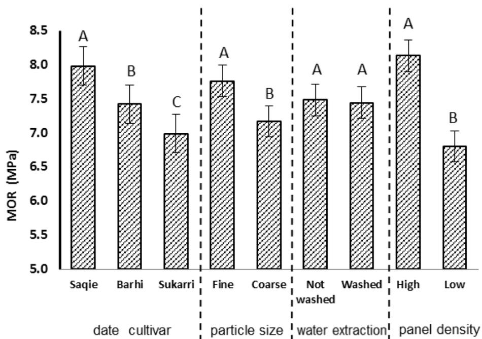
**Figure 5.** Effect of date palm cultivar, particle size, hot water extraction, and panel density on Modulus of Rupture (MOR) property. (Means with same letter do not significantly different at L.S.D.<sub>0.05</sub>).
