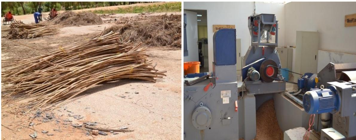
**Figure 1.** Date palm fronds without leaflets and the ring flaker machine (BX-466).
