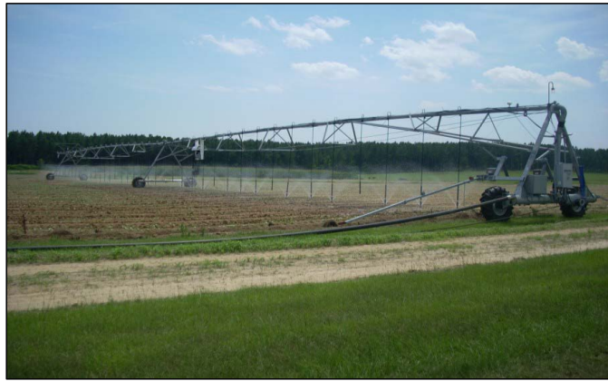
Figure 1. A 76-m linear move irrigation system used in these field studies [17].
