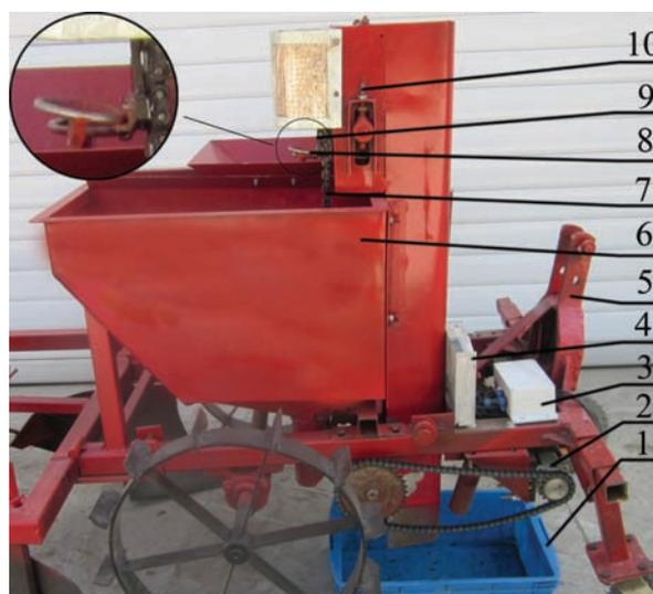
1. Collecting box 2. Motor 3. Controller 4. Driver 5. Frame 6. Seed box 7. Chain 8. Seed cup 9. Guard plate 10. Tightener
